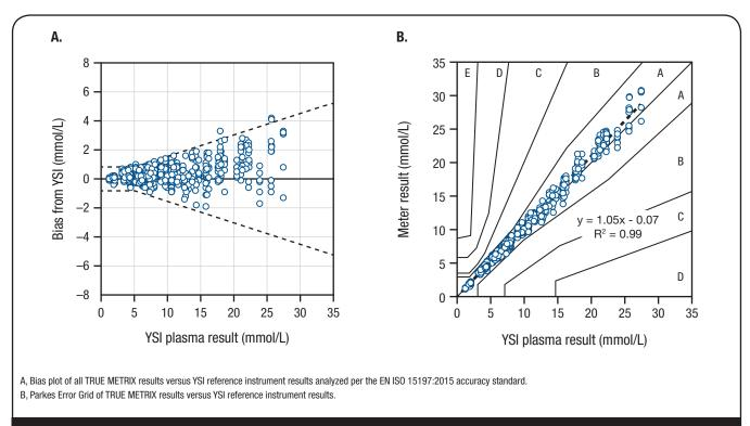
Figure 2. EN ISO 15197:2015 Accuracy Results for Healthcare Professionals Using TRUE METRIX Versus YSI Reference Instrument
